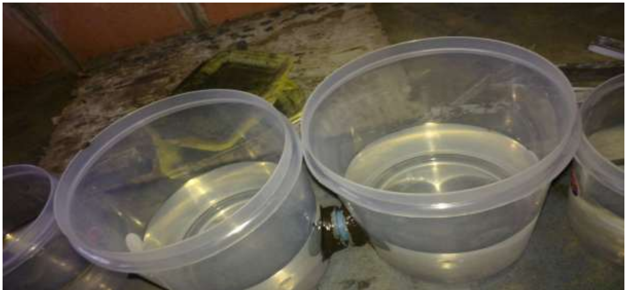
Figure 3: connect salt bridge with two plastic bottles and the use epoxy
