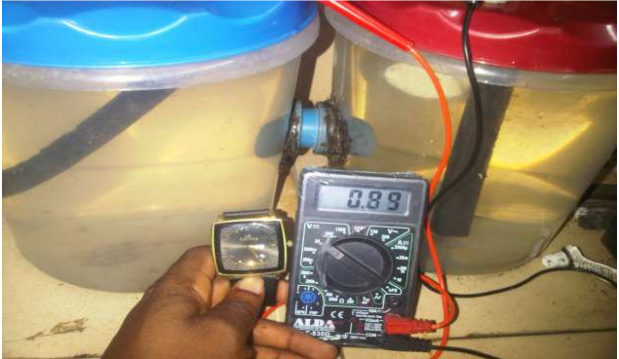
Figure 3:1. Photograph showing voltage taken on the 14 th day from cell
