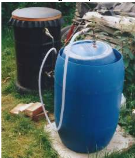
Figure 3: Biogas Construction for Methane Generation from cow Dung.
